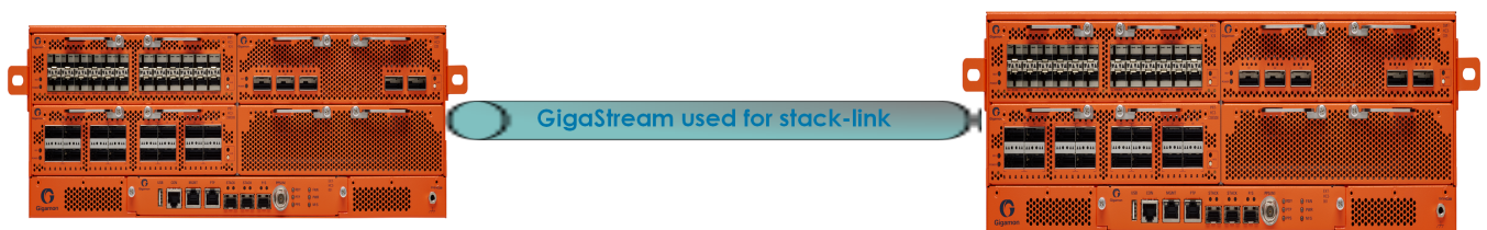
Figure 4 Daisy-Chain Configuration using GigaStream for Stack-link
